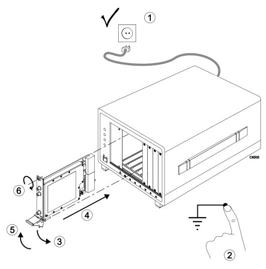
Fig. 5 Installing module into chassis (this procedure applies to any module)
