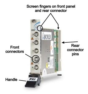
Fig. 1 Points to check for damage
