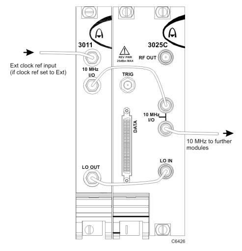
Fig. 6 Example of LO and 10 MHz connections
