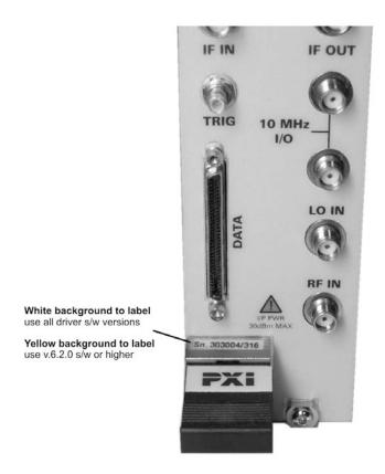
Fig. 4 Location of serial no. label (example)
